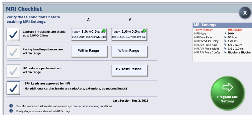
Figure 4. An example of the MRI Checklist screen for ICDs on the Merlin PCS
